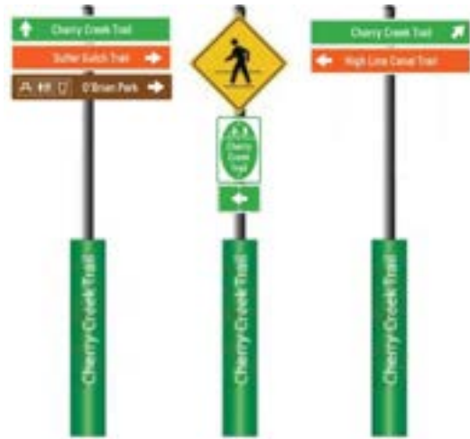
Directional sign examples that would integrate MUTCD signs, the on street network and the color scheme proposed in the Cherry Creek Trail Guidelines
